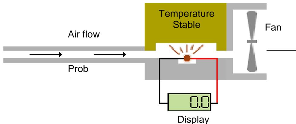
When gases with different thermal qualities pass through the chamber the amount of heat being transmitted to the Temperature Stable block changes. These changes are measured, calculated and displayed on GasCheck G as leak rates or gas concentrations.
