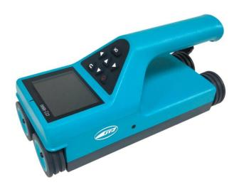
The integrated rebar detector is a portable non-destructive testing instrument, which can be used to test the construction quality of reinforced concrete structures. It can measure the position of rebars on the concrete surface, detect the thickness of the steel protective layer and the diameter of the rebar.
